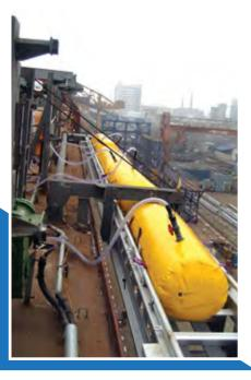
**Alatas** supplies certified water bags and calibrated load cells for Lifeboat, Davit System, Gangway & Accommodation Ladder testing.
